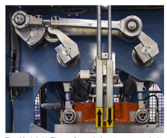
The Model 44 Thermoformer's key to success is its flexibility and adaptability. It provides exceptional performance throughout a range of sheet types, including TFPP, PP, PET, CPET, HIPS, and polystyrene foam. The optional Mini-Magnum configuration allows a 6" product depth making it an excellent candidate for cup production. Independent platen motion is on the Model 44 providing the timing necessary for processing shallow and deep products with the optimum of control.
