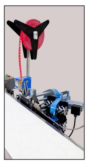
The MARK-60 bag closing system will bag 60 bags per minute using the Kwik Lok style clip (Optional I-LOK Clip). This system has three components that are in line that are mounted to a conveyor.
